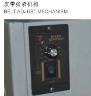
主轴进给速度无机可调 THE SPEED OF SPINDLE FEEDS INFINITELY ADJUSTABLE
