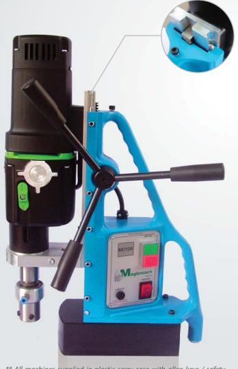
\*\* All machines supplied in plastic carry case with allen keys / safety chain with carabina hook / coolant system and drill drift MT 3 all models available in 110/120 Volts 50/60Hz and 220/240 Volts AC 50/60Hz
